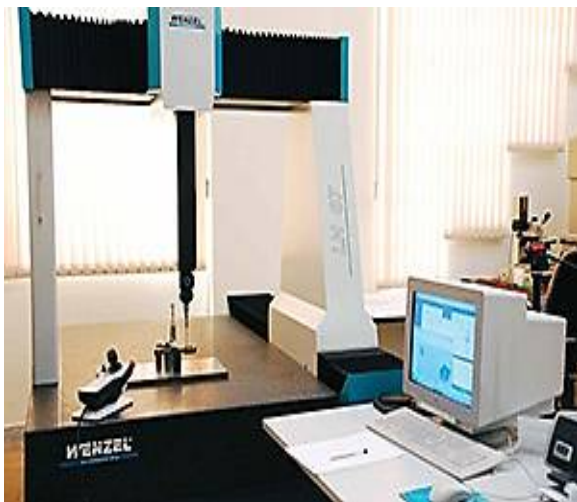
Fig. 2 The measurement of distortion with CMM.
