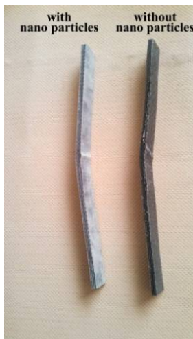
Fig. 8 Composite samples after bending test
