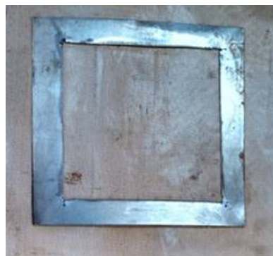
Fig. 1 Applied steel mold with the dimensions of 150x150x1 mm
