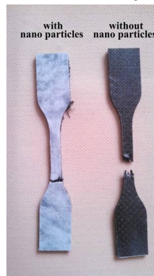
b) Composite samples after tensile test
