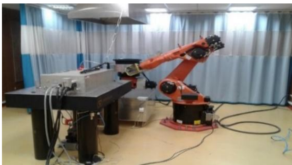
Fig. 2 The laser device and Six degrees of freedom robot Koka used in the research
