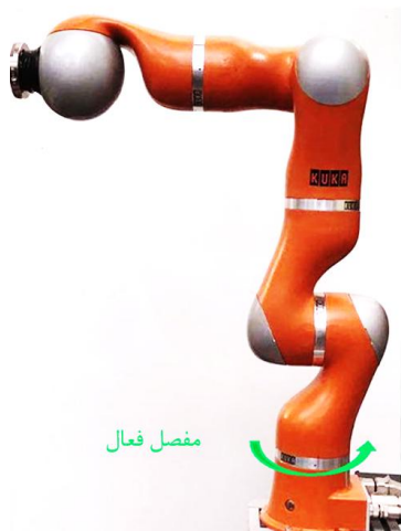
Fig. 5 First joint of the KUKA Light Weight IV robot is used as active joint in the experiments [12]
