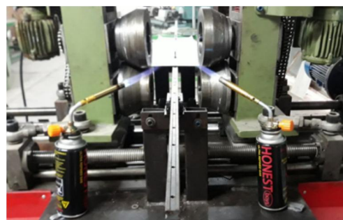
Fig. 10 flexible roll forming device with additional heating function
