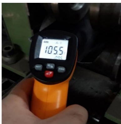
Fig. 11 Measuring sheet temperature with a laser thermometer
