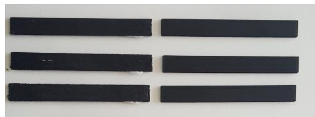
Fig. 10 Specimens made for three-point bending test
