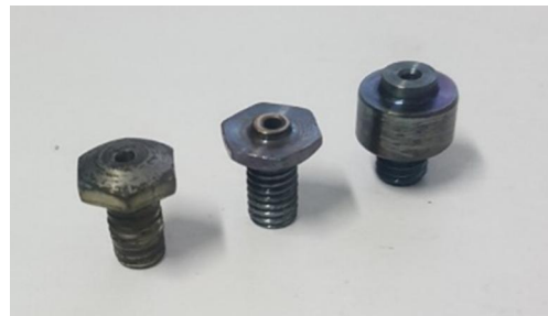
Fig. 7 Nozzles produced and suitable for printing with continuous fibers
