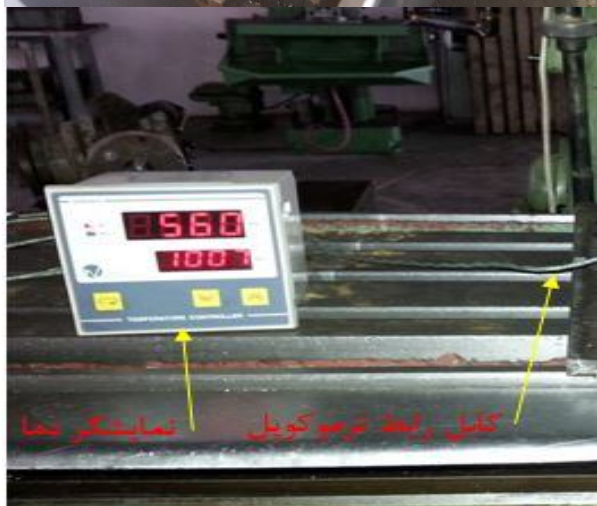
Figure 3 Conducting the operation of the friction-stirring process and recording the temperature of the work piece
