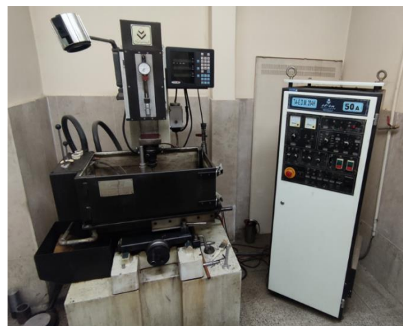
Fig. 3 Azarakhsh machine manufactured by Tehran Akram company, model TA-E.D.M.204H
