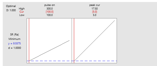
Fig. 13 Optimizing the process in terms of surface roughness
