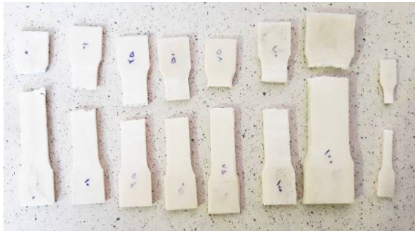
Fig. 7 The prepared printed specimens after tensile test.
