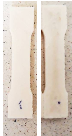
Fig. 5 Two printed specimens with different layer setup.
