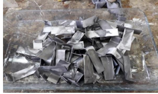
Fig. 5 Aluminum parts after reaction with sodium hydroxide
