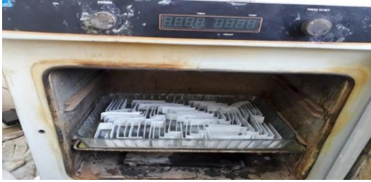
Fig. 6 Samples are placed inside the furnace after surface treatment for drying
