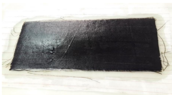
Fig. 4 Surface preparation of multilayer composite with Dacron fabric
