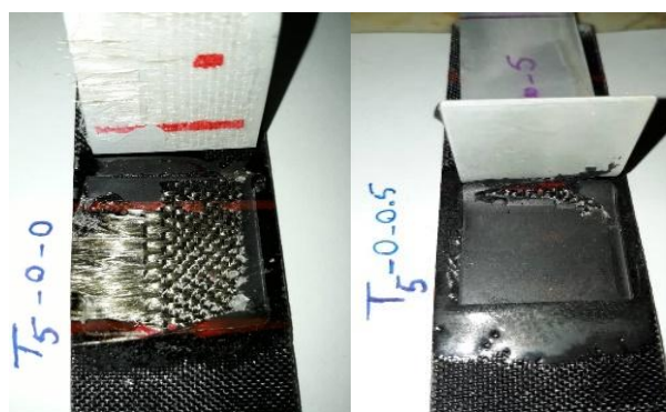
Fig. 22 Photo of T5-0-0 and T5-0-0.5 junction failure area
