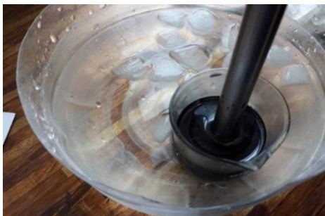
Fig. 9 Ice bath to keep the resin temperature low
