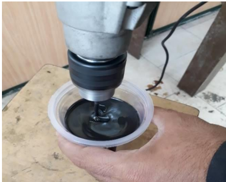
Fig. 7 Mechanical stirrer for mixing nano and resin
