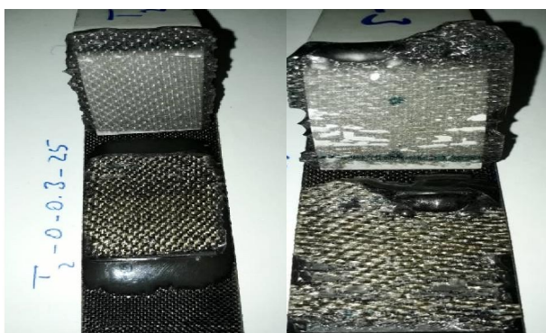
Fig. 28 Photo of junction failure area T-0-0.3-30 and T-0-0.3-30
