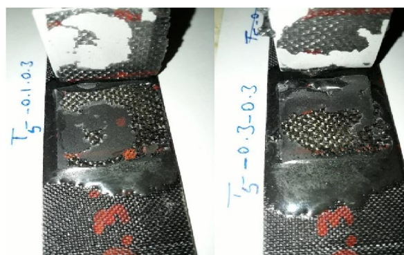
Fig. 23 Photo of T5-0.1-0.3 and T5-0.3-0.3 junction failure area
