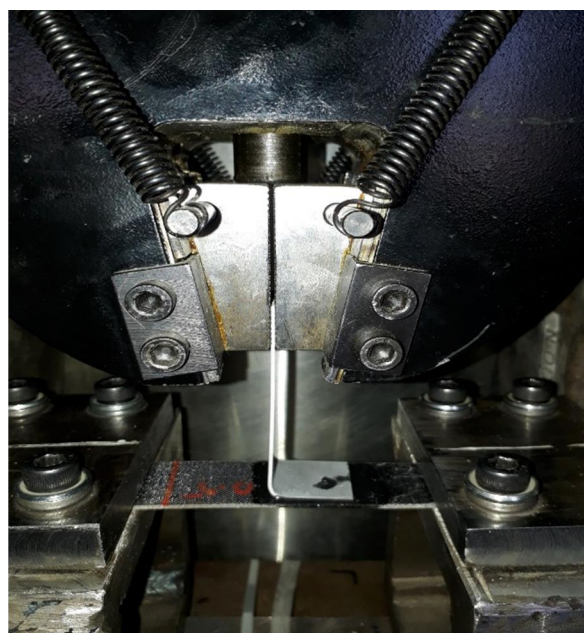
Fig. 12 How to test the tensile strength of L-shaped connection specimens
