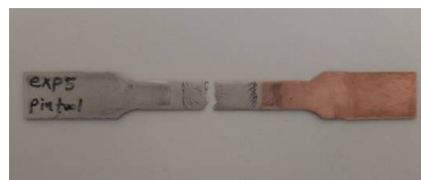
Fig. 5 Tensile test sample after failure
