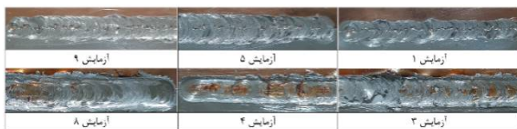
Fig. 9 Defective joints made with pinless tools
