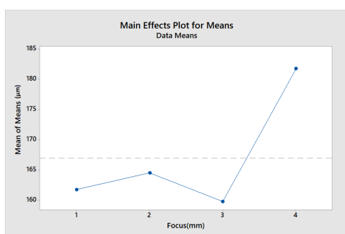
Fig. 14 The average depth of the HAZ relative to the focal length
