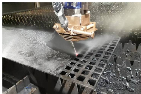
Fig. 2 The hybrid laser- waterjet process on CK75
