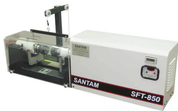
Fig. 3 View of Rotary fatigue bending test machine
