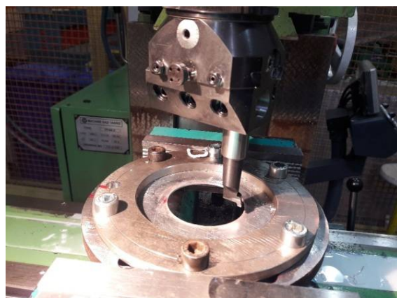
Fig. 2 Method of locating the fixture on milling machine table and drilling of sheet
