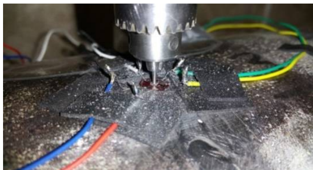
Fig. 2 overview of the residual stress measurement with hole drilling method
