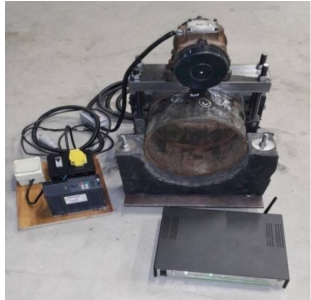
Fig. 3 Vibration stress relief setup on pipe
