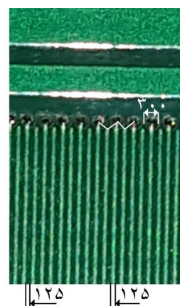
Fig. 8 Close up of for-phase electrodes. Sizes are written in micrometers
