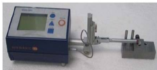
Fig. 2 Roughness measurement of the samples Taylor Hobson (model Surtronic-25)
