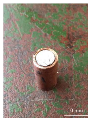
Fig. 1 Two-layer rod for hot forward extrusion
