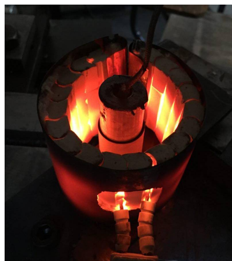
Fig. 3 Experimental setup of hot forward extrusion consists of the die, furnace and fixture
