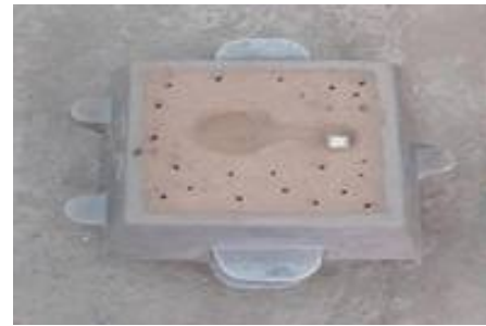
Fig. 4 Foam pattern at the mold box
