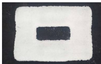
Fig. 13 One sample tested by the SLS machine with a 12-degree polyamide powder
