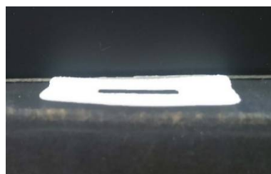
Fig. 12 Hollow rectangular side view to measure distortion
