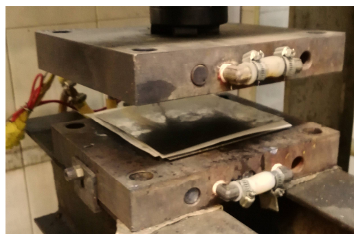
Fig. 2 Forming the PU/PCL blend with hot press set-up
