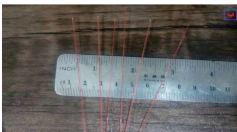
Fig. 1 Glass micro-tubes, a) before and b) after being filled by self-healing agent
