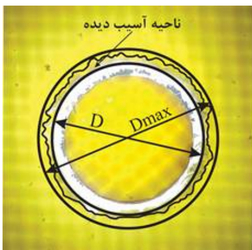
Fig. 4 Delamination zone, its diameter and nominal hole diameter
