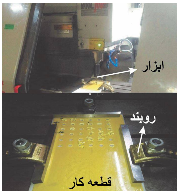
Fig. 2 Experimental tests implementation and composite sheet clamping
