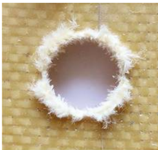
Fig. 5 Uncut fibers created in Kevlar/epoxy composite drilling
