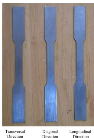
Fig. 6 Standard specimens of the sheet in three directions: longitudinal, diagonal and transversal
