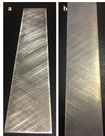
Fig. 1 Surface treatments on 2024-T3 aluminum sheets (a) mechanical treatment (b) mechanical and chemical treatment
