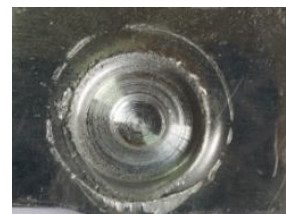
Fig. 7 Distortion of sheet in tool rotational speed of 2000 rpm
