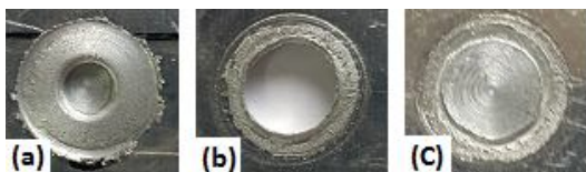
Fig. 8 Different regions of joint in tool plunge depth of 1.4 mm (a) schematic of joint (b) lower surface of the upper sheet (c) upper surface of the lower sheet
