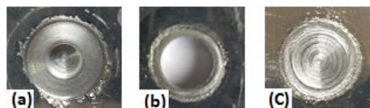
Fig. 6 Different regions of joint in tool rotational speed of 625 rpm (a) schematic of joint (b) lower surface of the upper sheet (c) upper surface of the lower sheet
