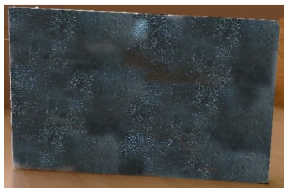
Fig. 3 Composite sample manufactured with delamination defect
