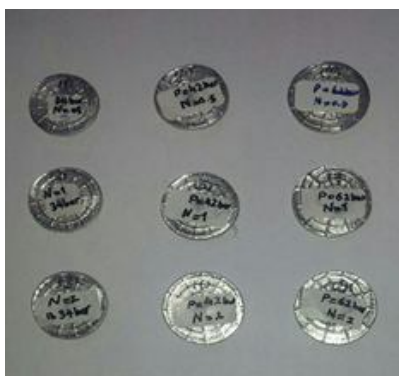
Fig. 2 The obtained disks from unconstrained HPT process
