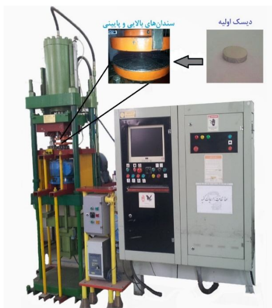
Fig. 1 Unconstrained HPT's machine
