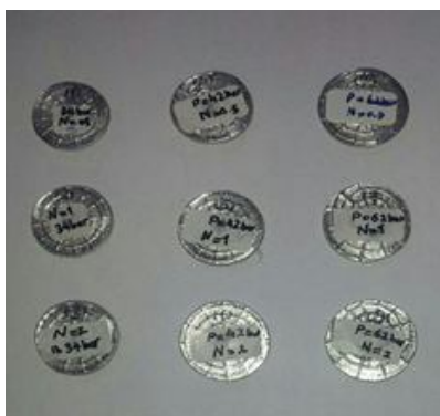
Fig. 2 The obtained disks from unconstrained HPT process
