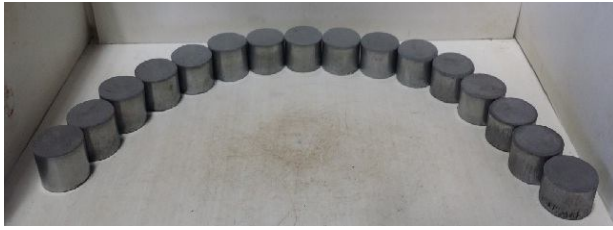
Fig. 4 Samples fabricated using dynamic compaction method
