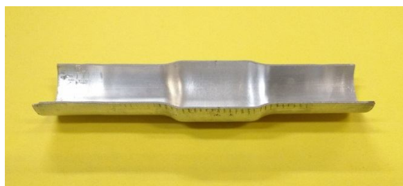
Fig. 7 A cut sample with marked edge for thickness measurement
