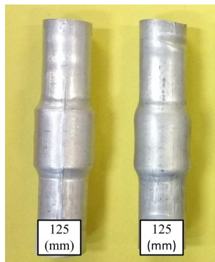
Fig. 11 Rubber-pad bulged samples with same initial length of 125 millimeters and with L125 (right) and L125-modified (left) loading curves
