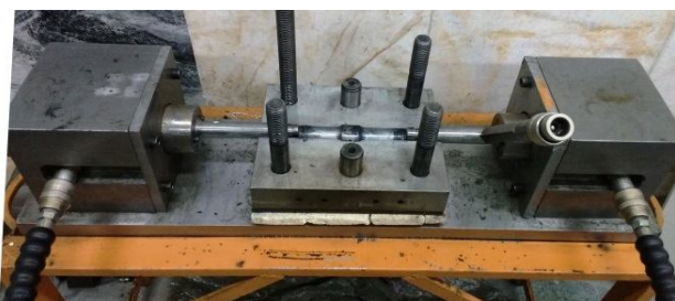
Fig. 2 Experimental setup used for rubber-pad bulging
