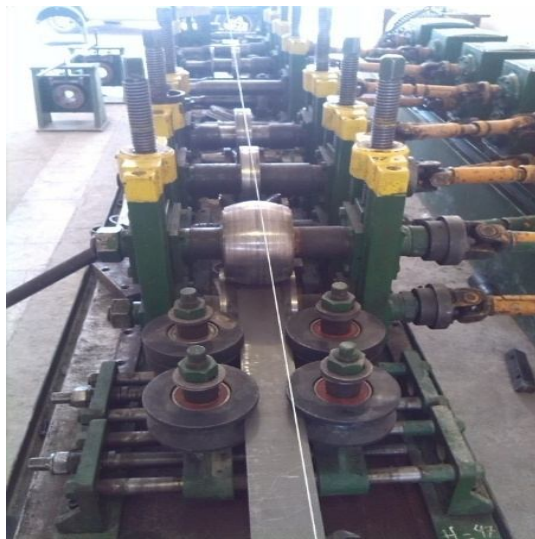
Fig. 6 Cold roll forming machine used in experiments
