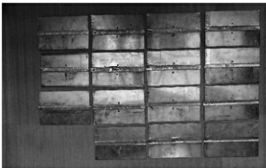
Fig. 3 Welding samples with a thickness of 1.8 millimeters
