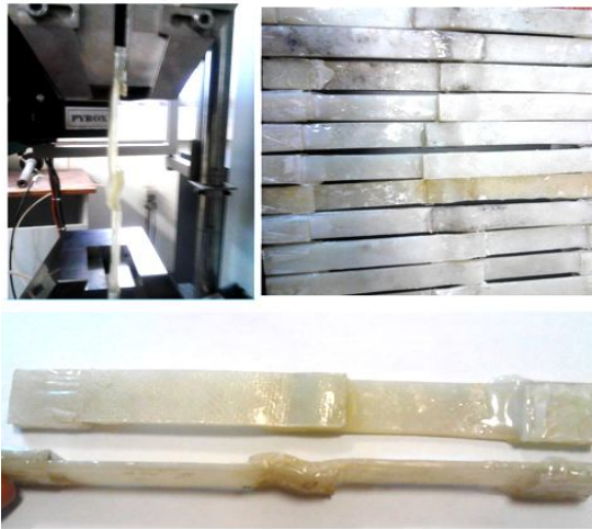
Fig. 3 Prepared Specimens and tension test
