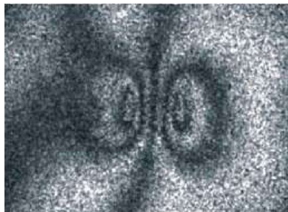
Fig. 6 Fringe pattern obtained in an experiment with load F=294 \text{N}
