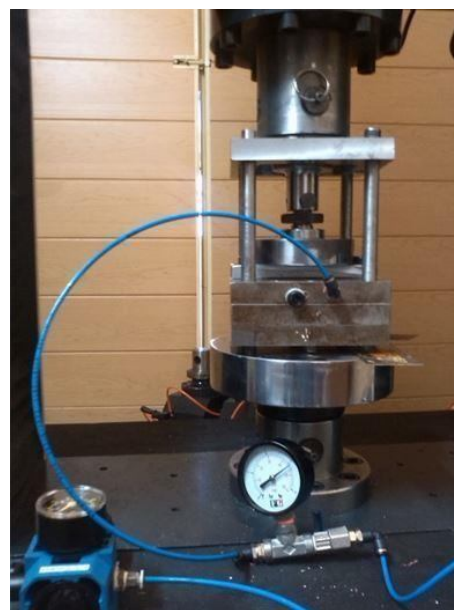
Fig. 1 A view of a system designed to measure the amount of leakage
