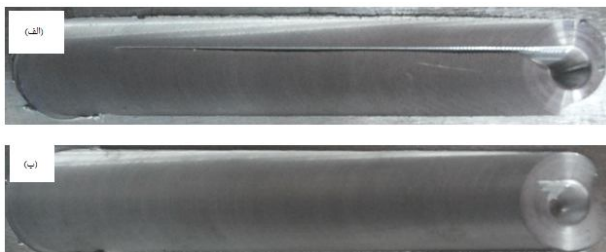
Fig. 16 Surface material flow in joint which welded by (a) 0.2 and (b) 0.4 mm tool plunge depth
