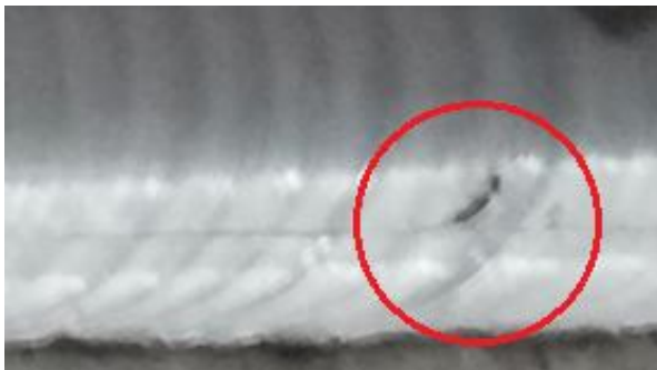
Fig. 8 Surface defect which formed in joint with 108 mm/min travelling speed
