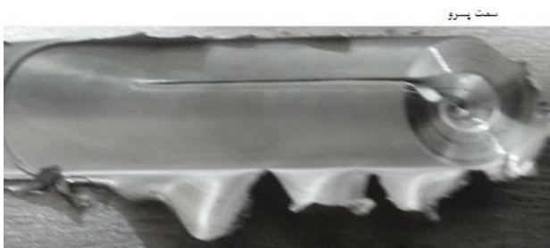
Fig. 6 Side flash on joint surface
