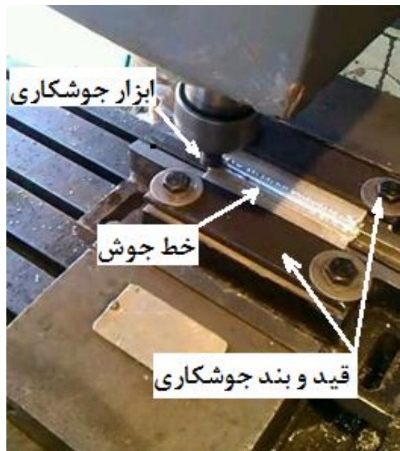
Fig. 3 FSW tool in welding progress
