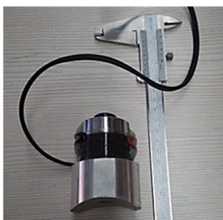
Fig. 2 100 watts transducer with concave cross-section
