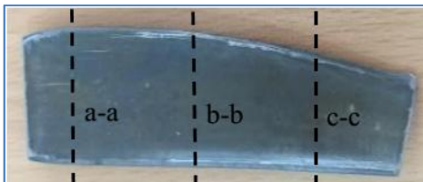
Fig. 22 Sample of baffles produced by hydroforming method
