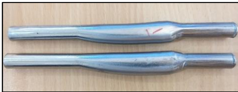
Fig. 18 Preformed pipes of AISI304 stainless steel material
