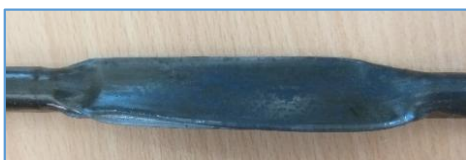
Fig. 20 Final hydroforming pipe at 200 bar oil pressure
