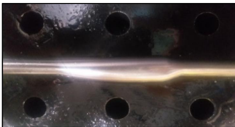
Fig. 19 Preformed pipe in preform mold
