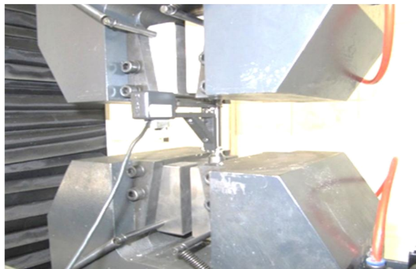
Fig. 4 Tension test sample in Santam Machine
