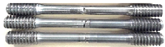
Fig. 8 Failure of the samples from the weld
