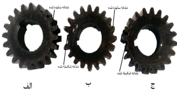
Fig. 4 A-Gear with a fractured tooth, B-Gear with a fractured and a worn tooth, C-Gear with a worn tooth
