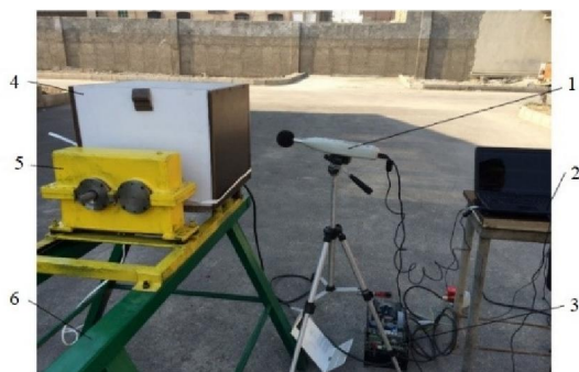
Fig. 2 Components of the fabricated system: 1-Sound level meter, 2-Laptop computer, 3-Inverters, 4-Electromotor acoustic chambers, 5-Gearbox, 6-Chassis
