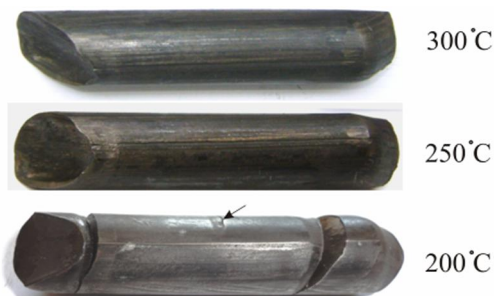
Fig. 4 Appearance of CP-Ti samples after single pass of ECAP by pressing speed of 1 mm/s at different processing temperatures
