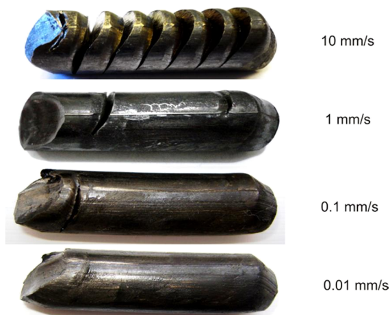
Fig. 5 Appearance of CP-Ti samples after single pass of ECAP at 200 °C and using different magnitudes of pressing speed. The numbers shown next to the samples indicate pressing speed
