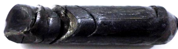
Fig. 6 Appearance of CP-Ti sample after second pass of ECAP at 200^\circ\text{C} and using pressing speed of 0.01 \text{ mm/s} . The second pass was conducted using route B C
