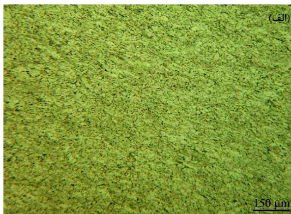
Fig. 7 Light microscopy micrographs taken from the longitudinal sections of CP-Ti samples after processing by single pass of ECAP at 200^\circ\text{C} : (a) The region between two cracks and away from the opening of cracks in the sample ECAP-ed by pressing speed of 10 \text{ mm/s} , (b) The region near the opening of crack in the sample ECAP-ed by pressing speed of 10 \text{ mm/s} , (c) The region between two cracks and away from the opening of cracks in the sample ECAP-ed by pressing speed of 0.1 \text{ mm/s} , (d) The region near the opening of crack in the sample ECAP-ed by pressing speed of 0.1 \text{ mm/s}
