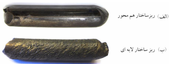
Fig. 10 Appearance of CP-Ti samples by different initial microstructures after single pass of ECAP at 250 °C and using pressing speed of 1 mm/s: (a) the sample with equiaxed initial microstructure (b) the sample with lamellar microstructure
