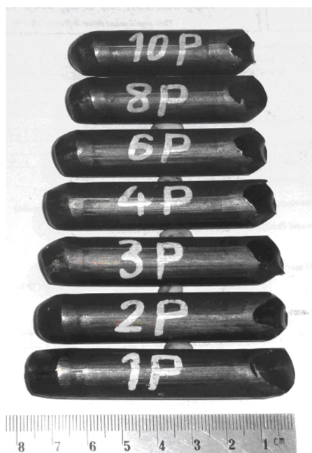
Fig. 12 Appearance of CP-Ti samples ECAP-ed at 250 °C for different number of passes and using pressing speed of 1 mm/s. 1P, 2P, ..., 10P indicates respectively the number of passes from 1, 2, ..., 10 applied on samples
