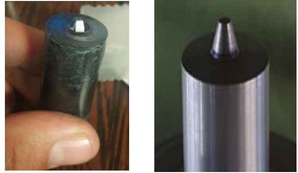
Fig. 2 Cylindrical tungsten carbide tool pin with circular and square cross section
