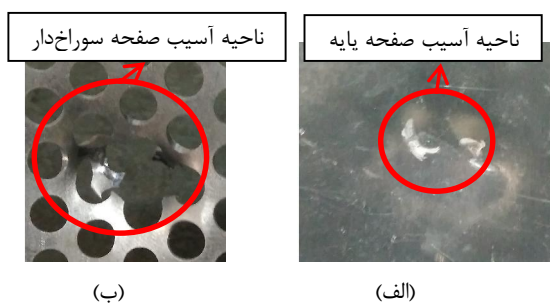
Fig. 16 Experimental study – distance of two plates less than the length of the projectile (a- base plate, b- perforated plate)
