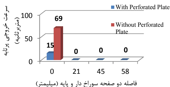
Fig. 18 Projectile output velocity in presence / absence situation of perforated plate
