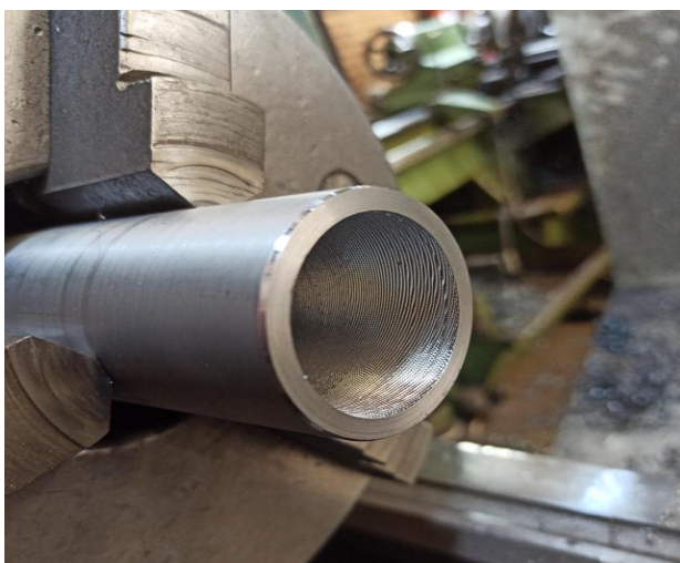
Fig. 2 The low surface quality of workpiece due to excessive boring bar vibration
