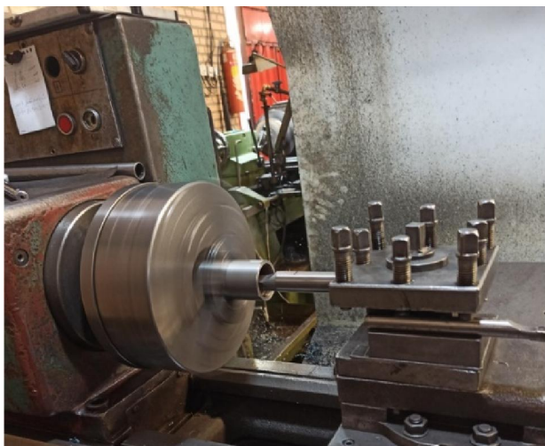
Fig. 1 Boring bar tool during boring operation
