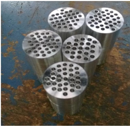
Fig. 1 The sample of the primary work piece that is placed in the melting furnace
