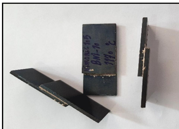
Fig. 3 10 min Brazed specimen following brazing process
