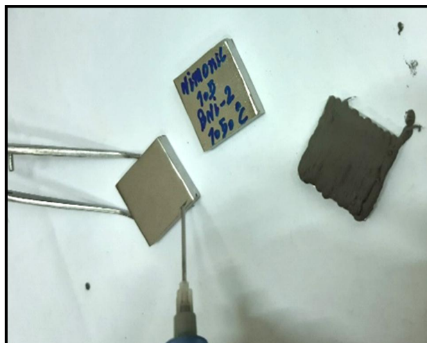
Fig. 2 Applying the BNI-2 filler in the form of paste to base metals
