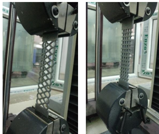
Fig. 6 A picture of how the samples are placed in the tensile test machine
