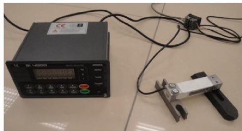
Fig. 5 Load cell with display for force measurement
