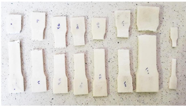
Fig. 7 The prepared printed specimens after tensile test
