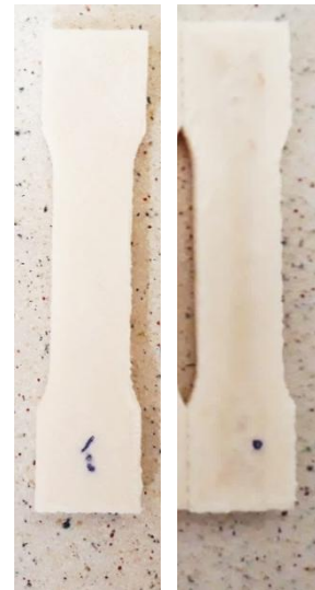
Fig. 5 Two printed specimens with different layer setup
