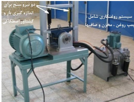
Fig. 8 The test device was built to evaluate the functional characteristics of the bearing
